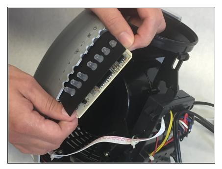
• Locate the control board and grab it by the top and bottom firmly. Pull the board straight out being careful not to flex the circuit while removing.
