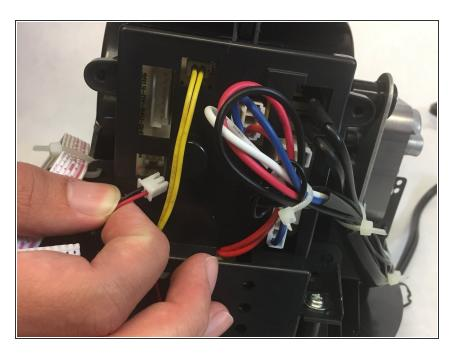
• Unplug 2 pin wires which connects the front LED's.
