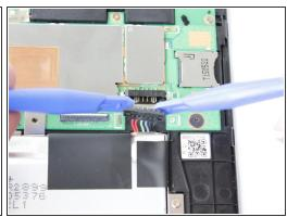
Remove the battery connector by prying it up away from the device using 2 plastic pry tools
