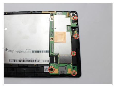
Using the #00 Phillips head screwdriver, remove the remaining 1.5mm screws in the motherboard
