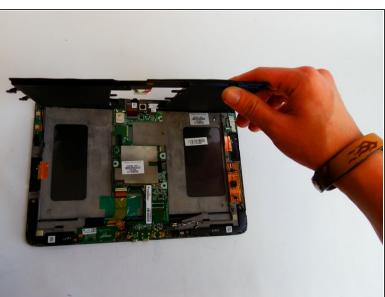
Lift the battery up by its edges and remove it carefully. There will be adhesive holding the battery down.
