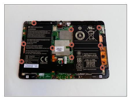
Unscrew the ten 3.3 mm screws securing the battery using a 00 Phillip's head screwdriver.
