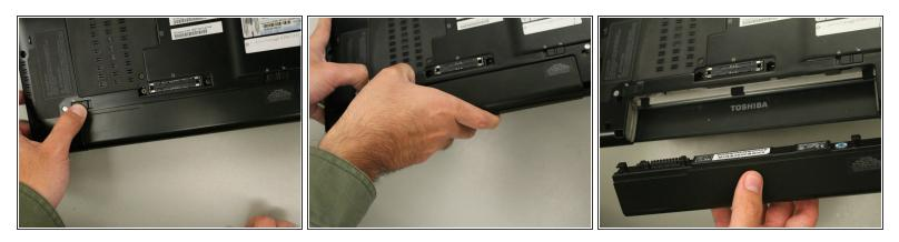
• Hold the next lock in the unlock position. Simultaneously pull the battery towards you.
