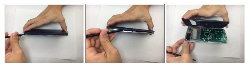
• Use plastic spudger to separate backplate from the front-plate. Place the flat end of the spudger in the seam between the front and back, near one end of the calculator. Then slide the spudger towards the calculator's center. The two sides will pop free from each other as you go through it with the spudger.
