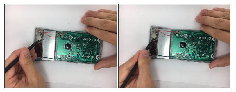
Using the pointed end of the nylon spudger, carefully pry an edge of the battery, and lift the battery from its socket.
