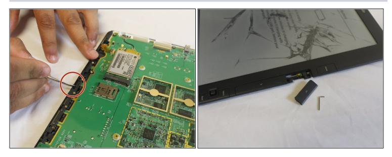
• Remove the "previous page" button from the side function keys using a pair of tweezers.
