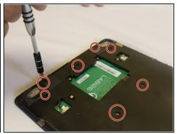
Remove five 30 mm screws from the midframe using a Phillips #000 screwdriver.
