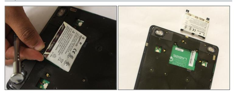
Remove the battery from the device.
