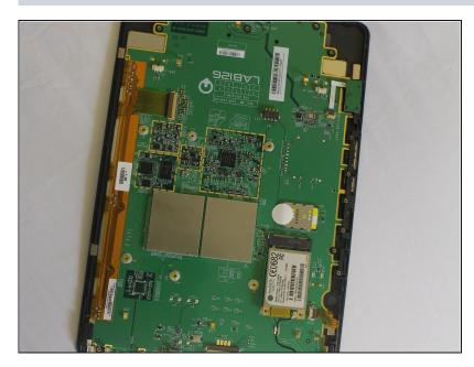
• Remove the midframe to reveal the motherboard.
