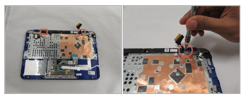
• Remove the two screws that hold down the LCD hinges.
