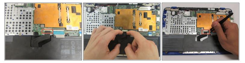
Use your fingers (or a set of tweezers) to disconnect the battery cable from the motherboard by gently pulling it towards the battery.
