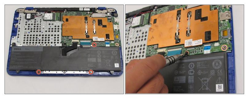
• Use a Phillips screwdriver to unscrew the three 4 mm screws securing the battery.
