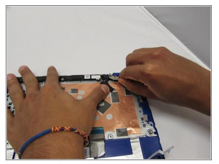
• Pull the hinges back and remove the screen.
