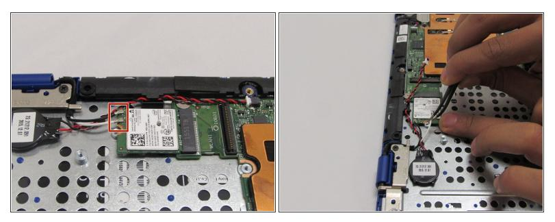
Using the tweezers, pull the white and black wires off of the WiFi Chip.
