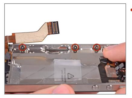
• Loosen the three large-headed Phillips screws along the other side of the iPhone about one half turn.
