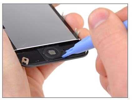
• Use the edge of a plastic opening tool to gently peel the bottom right corner of the home button assembly from the display assembly.
