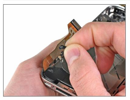
• Remove the small plastic bracket that was installed under the screw closest to the dock connector cable.
