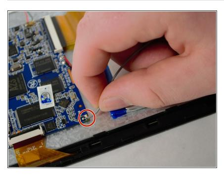
You can check one of the connection points between the battery and the motherboard to see if it is firmly connected (which it should be) using the plastic Spudger. It is not necessary to remove this wire to replace the battery.
