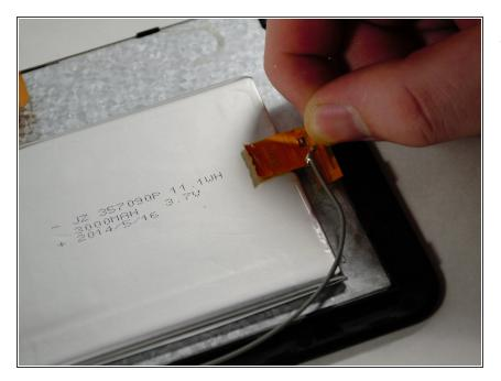
Use your fingers to separate the ribbon wire from the battery and the back of the display.
