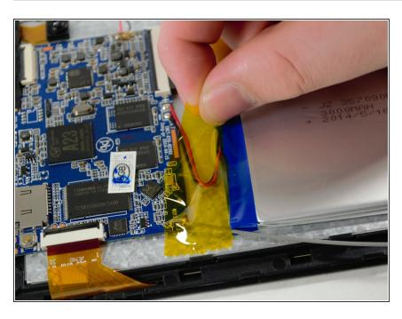
Use your fingers to remove more yellow tape holding down the wire connecting the battery to the motherboard.
