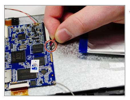
You may use the plastic Spudger to separate the connections between the battery and motherboard. The new battery is now ready to be soldered on.
