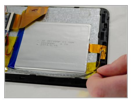
Remove the yellow tape holding the wire connecting the battery to the motherboard with your fingers.
