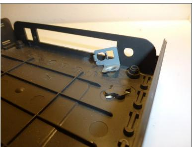
The last piece of the router is this small metal clip here. Simply pull it up.
