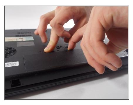
Slide and hold switch number 2 to the left, and use your finger to pry battery out using the slot to the right of the switch.
