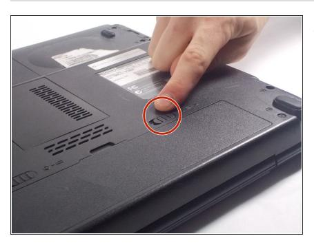
Make sure switch with the number 1 is moved to the right, in the unlocked position.
