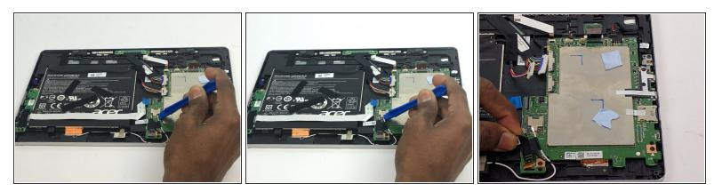
• Use your plastic opening tool to pry up and lift the antenna cables from the motherboard.
