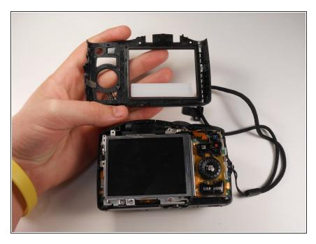
Remove back plate from the camera and locate the orange button plate to the right of the screen.
