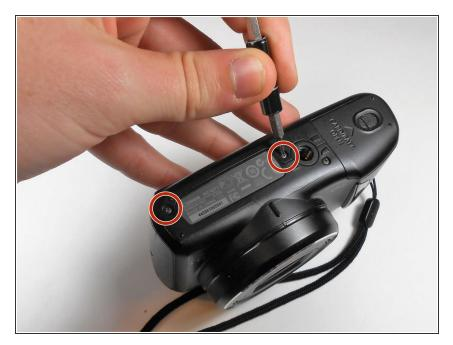
Remove the two, 4mm screws from the bottom of the camera. Continue using the same screwdriver from step 1.
