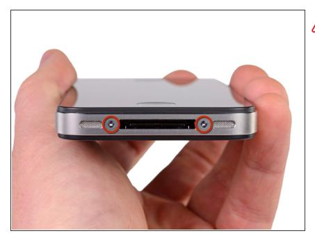
A Before you begin, discharge your iPhone battery below 25%. A charged lithium-ion battery can catch fire and/or explode if accidentally punctured.
