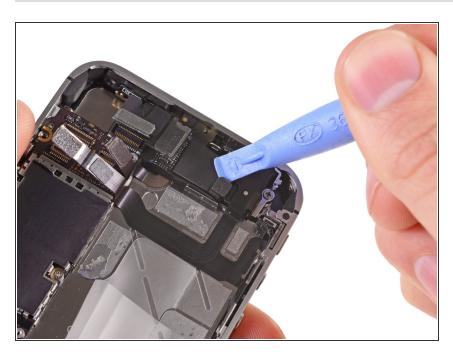
Use the edge of a plastic opening tool to disconnect the Wi-Fi antenna from the logic board.
