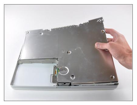
Lift the bottom shield off.
