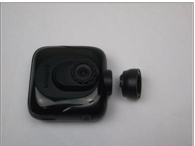
Remove the Dash Cam socket piece.
