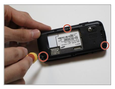
• Use a Phillips #00 screwdriver to loosen and remove all 3 screws.
