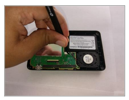
• Lift and separate the speaker connector cable using a pair of tweezers.
