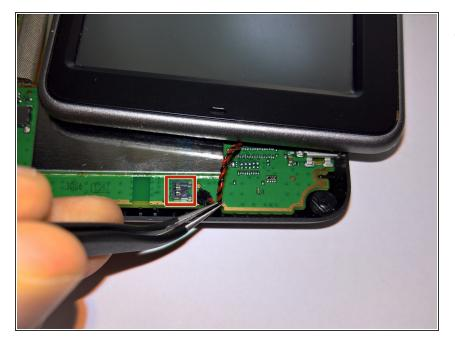
Lift the connector gently from the socket, making sure you pull in the right direction.
