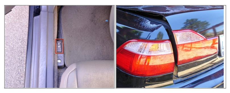
• Open the trunk using your key in the trunk key slot or by using the lever under the driver's console.
