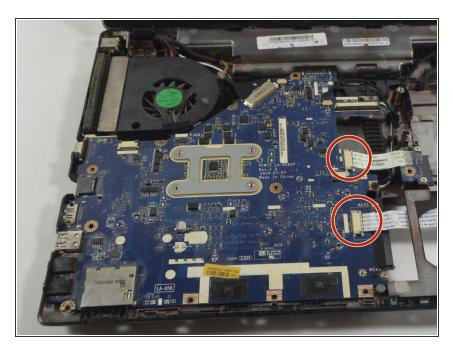
Remove the two remaining ribbon cables as described in Step 11.
