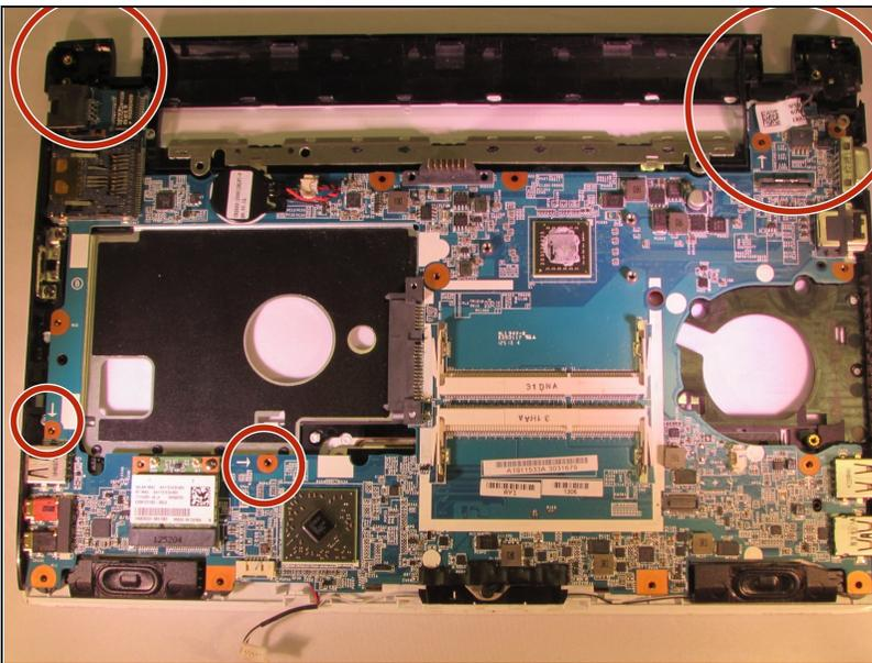
● Locate and remove the screws holding the motherboard down.
