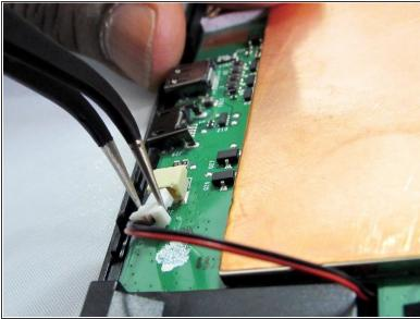
Remove the red and black wire connector from the motherboard using either fingers or tweezers.
