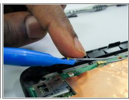
Remove both antenna connectors with a blue opening tool/tweezers.
