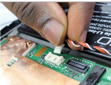
Remove the connector at the top of the motherboard by pulling the connector away from the motherboard with fingers or tweezers.
