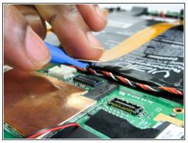
Remove the ribbon connector at the top of the motherboard using the opening tool.
