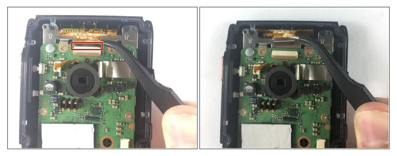
• Use precision tweezers to remove the connector joining the LCD and the motherboard.
