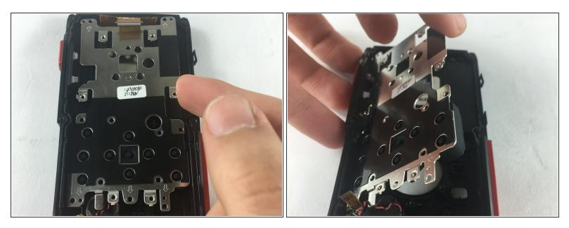
• Lift the metal plate by pushing it up from the top right edge of the plate.
