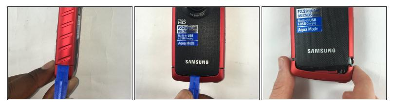
• Use the plastic opening tool to separate and remove the bottom red casing. Do this by, pushing the tool into the seam and prying up the red casing as you move along the edges.
