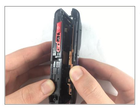
• Separate the front and back casing.
