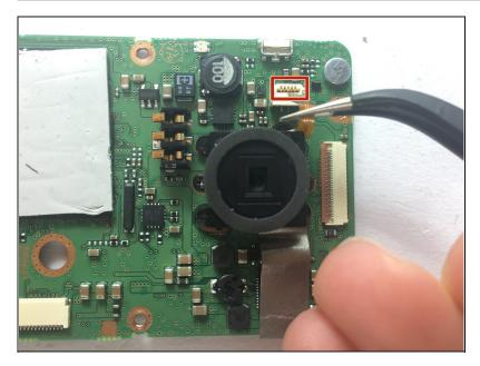
Use the precision tweezers, to gently pull and remove the connector connecting lens and motherboard.
