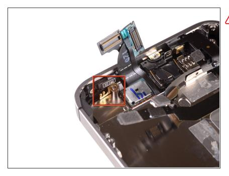
Be sure not to lose the small grounding finger for the rear facing camera near the power button. This finger rests on top of the PCB, screwed down, and covered with the adhesive black plastic tape.
