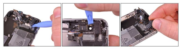
A In this step, be careful not to remove the headphone jack without first separating the top microphone from the upper case, as they are connected by a fragile flex cable.
