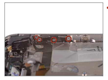
Remove the four 1.5 mm Phillips screws securing the volume button and silent switch brackets to the outer case.
