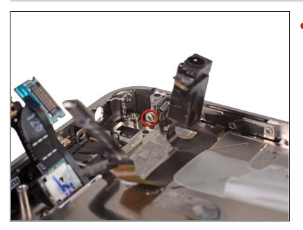
• Remove the 1.6 mm Phillips screw securing the mute switch bracket to the outer case.
