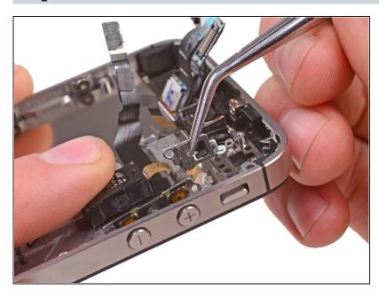
• Use a pair of <u>tweezers</u> to gently pull the silent switch bracket away from the outer case.
