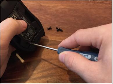
Use a Philips #0 screwdriver to remove the four screws that are keeping the mouse sensor assembly sealed.
