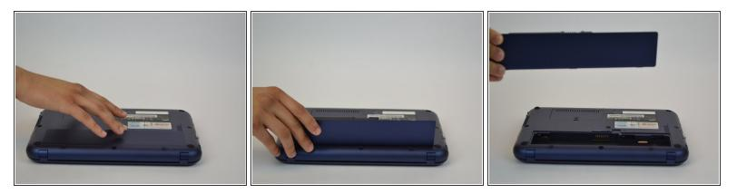
Make sure the laptop is powered off, and unplugged before removing the battery.
