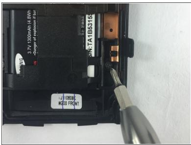
Remove the four 4.00mm screws holding the battery brace using a Phillips #00 screwdriver.
