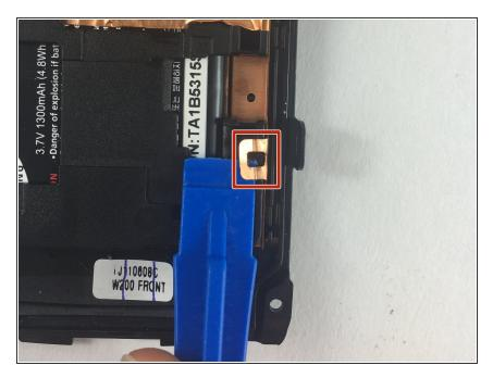
Using a plastic opening tool, lift the copper tab holding the battery brace in place.
