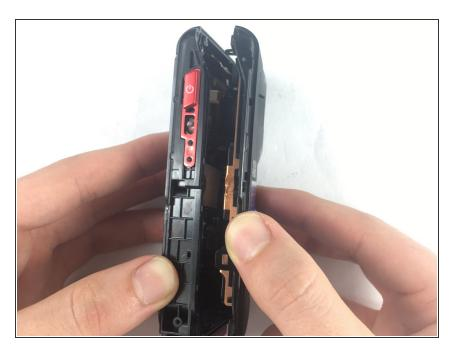
Separate the front and back casing.
