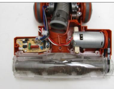
Use a Phillips #2 screwdriver to remove the four visible screws securing the rotary brush to the vacuum.
