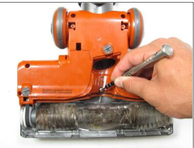
Use a Phillips #2 screwdriver to extract the three screws revealed from removing the plate.
