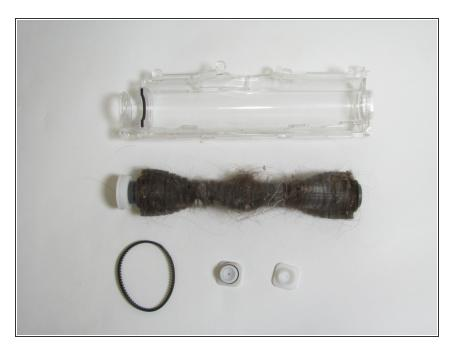
Remove the rotary belt attached to the brush and replace it if needed.
