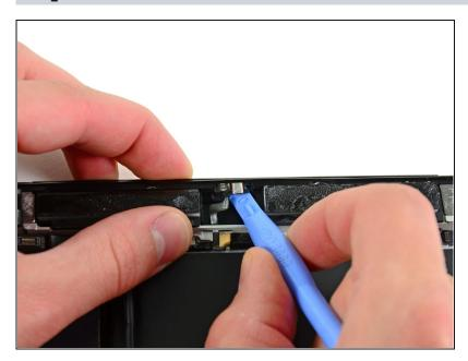
Carefully peel the microphone off the top edge of the rear panel.
