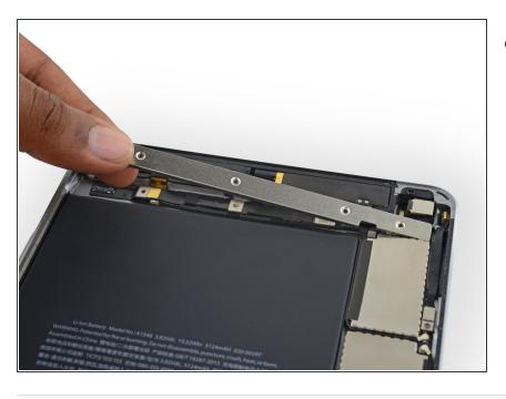
Remove the upper component cable bracket.
