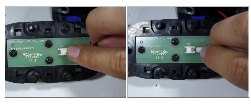
Firmly press on the end of the latch and pull the two-wire connector away from the base.
