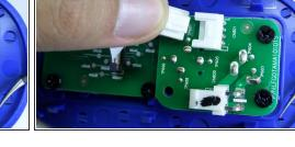
Firmly press on the end of the latch and pull the four-wire connector away from the base to separate.
