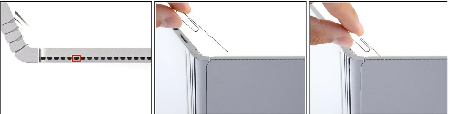
**i** The Surface Book has an internal lever arm mechanism that can be manually actuated through an access hole in the vents on side of the display.
