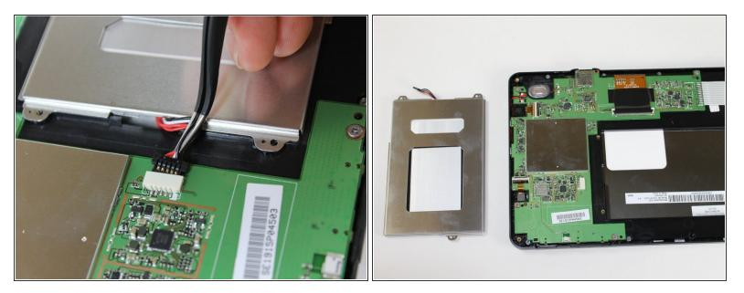
Unplug the battery and remove from device.
