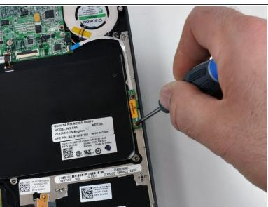
We believe this is an ambient light sensor to support the Adamo's backlit keyboard. Dell has used light sensors in a <u>few other</u> recent notebooks.
