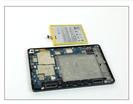
Remove battery from compartment and replace it with a new one.
