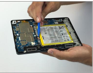
• Insert the plastic tool below the battery connecting wires and lift the tool to disconnect the wires from the device.
