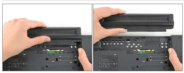
• Now push and hold the right switch to the right while using the other hand to gently slide the battery upwards out of the laptop.
