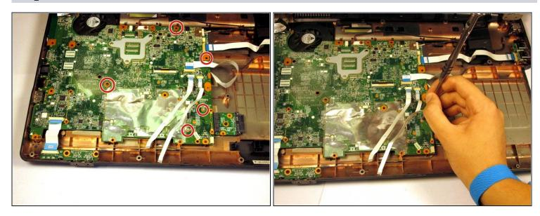
• Remove the five highlighted screws using a Phillips #0 screwdriver.
