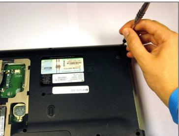
• Remove all fourteen 6mm screws using a Phillips #0 screwdriver.
