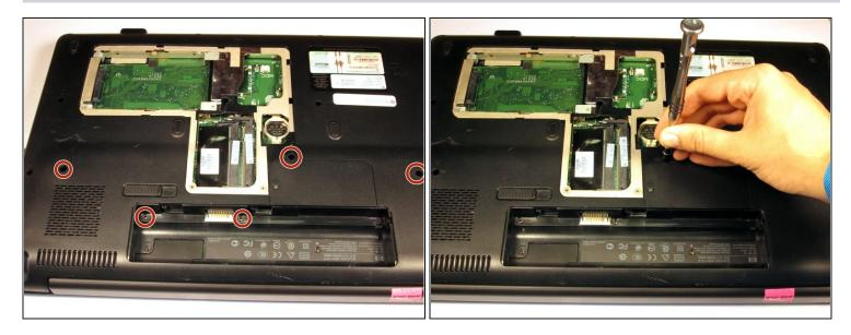
• Remove the five 6mm screws with the Phillips #0 screwdriver.
