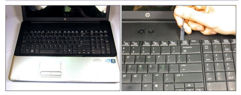
Pry the keyboard off with a spudger. Be careful not to apply too much pressure and damage any components.
