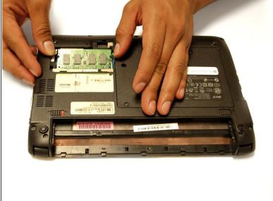
Using two fingers, gently spread the latches on the sides of the RAM card until the RAM card props up.
