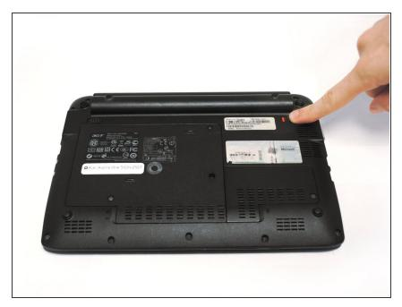
To unlock the battery, slide the lock latch in the direction indicated by the unlocking icon. You should see the orange indicator which means that the latch is unlocked.
