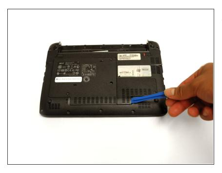
Use the plastic opening tool on the recessed notch at the bottom of the small plate to gently lift the plate up
