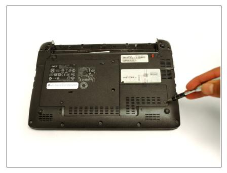
Use the #0 Phillips Screw bit with the Screwdriver to remove the single 6mm Phillips screw from the small back plate.
