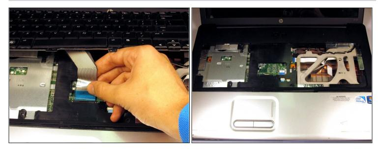
• Disconnect the clip attaching the keyboard wiring to the motherboard. Lift and remove the keyboard.
