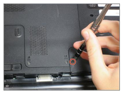
• Remove the 6mm screw from the cover above the battery using a Phillips #0 screwdriver.
