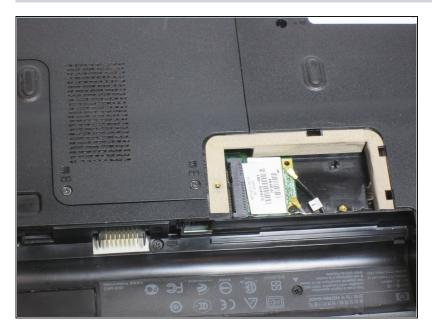
• Pull off the bottom cover to reveal the Wi-Fi card.
