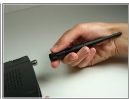
Unscrew each of the antennas from the wireless device.
