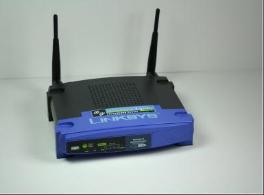
Once the old antennas are removed, replace them with them with the new ones by screwing them on the device.
