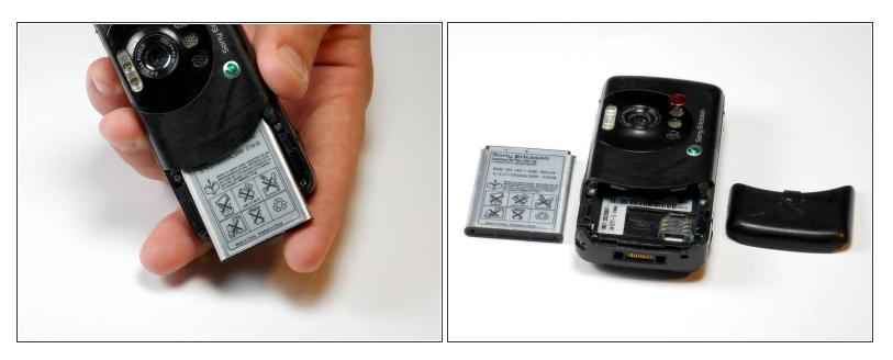
• Lift the bottom of the battery away from the phone with your thumb and rotate until the opening in the bottom of the case is oriented downward. The battery should slide out.
