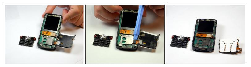
Insert the plastic opening tool under the ribbon cable attachment and give a small push upwards to dislodge it.
