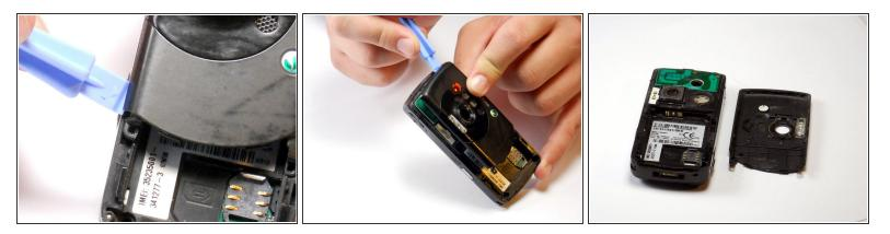
• Run a plastic opening tool along the edge of the back casing while prying it apart to remove it.
