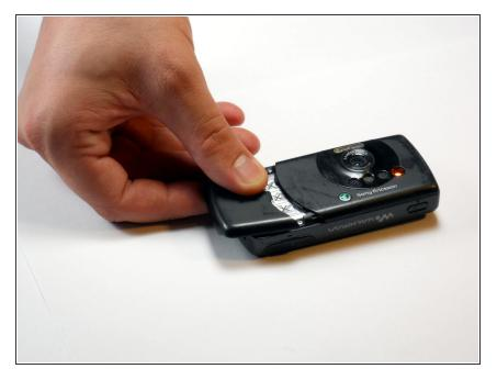
Remove the battery cover by applying downward pressure on the Singular Symbol and then shifting the pressure towards the bottom edge of the phone.
