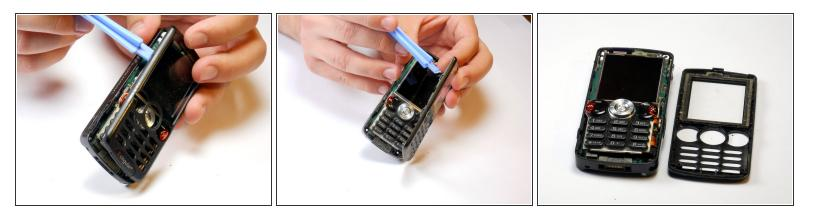
• Run the plastic opening tool upwards along that side, removing the housing.
