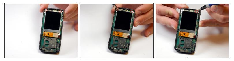
• Remove the indicated 6.35mm screws with a Torx T6 screwdriver.
