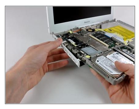
Lift up the left side of the computer and slide the I/O bezel away.
