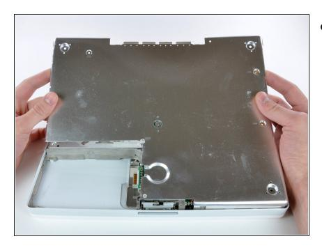
• Lift the bottom shield off.
