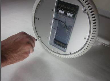
Remove the four 25mm T-15 screws.
