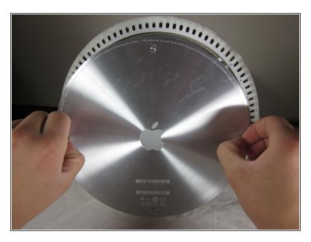
Carefully remove the base access panel.
