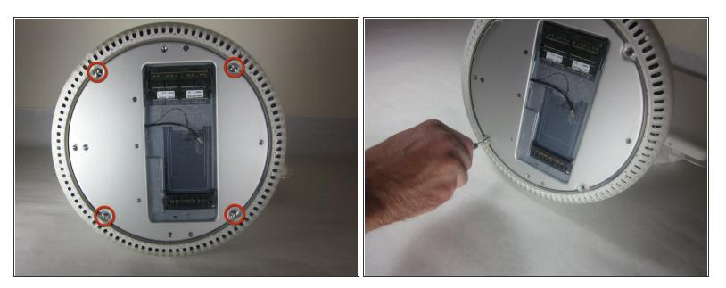
Remove the four 25mm T-15 screws.
