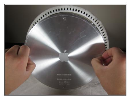
• Carefully remove the base access panel.
