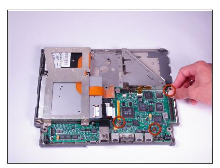
Remove the three cylindrical silver spacers placed on top of the motherboard.
