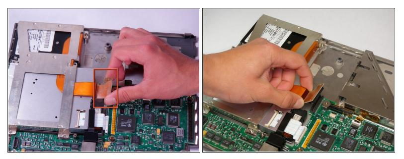
• Lift up on the orange connector attached to the hard drive until it releases from the motherboard.
