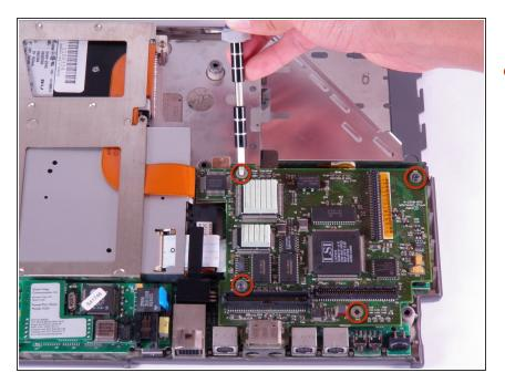
Use T8 torx screwdriver to remove four, 7.7mm long screws from the perimeter of the daughterboard.
