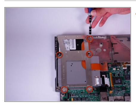
Use a T8 torx screwdriver to remove the five, 6.8mm long screws on the drive retainer.
