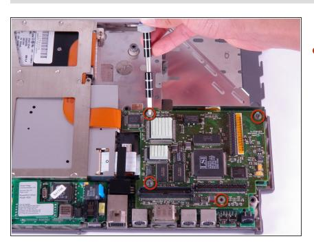
Use T8 torx screwdriver to remove four, 7.7mm long screws from the perimeter of the daughterboard.
