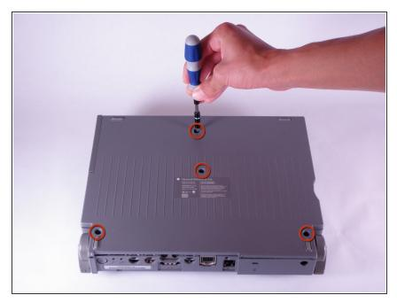
Use a T10 torx screwdriver to remove the four, 18mm long screws from the lower case.
