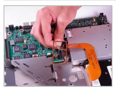
Pull the orange connector attached to the ribbon cable until the connector releases from the motherboard.
