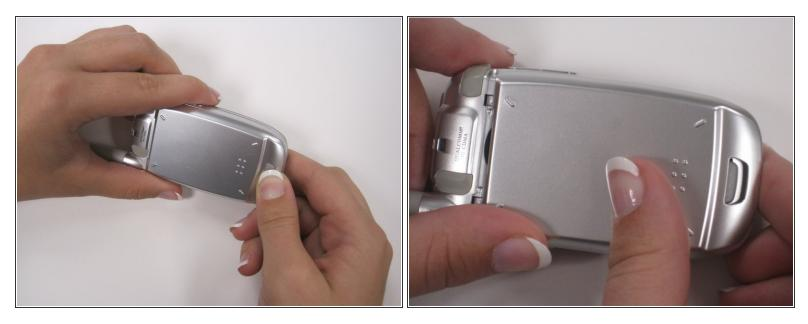
• Remove the back panel by first pressing and holding the gray button on the back. While doing that also press and slide the panel down and off.
