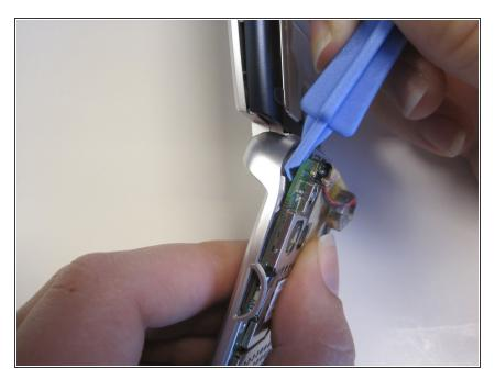
• Then use the plastic opening tool to remove the motherboard from the front half of the phone.
